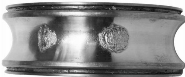
Fig. 4.1 Example of Flaking
